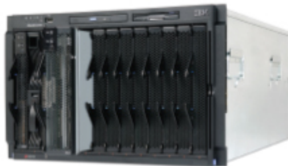
IBM BladeCenter Chassis with HS40 Blade Server
